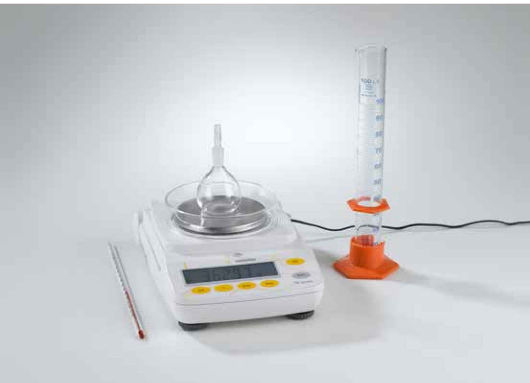
Determination of density with the pycnometer (C3.1.2.4)
